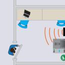
Presence is detected and the device logs this against a date and time,
